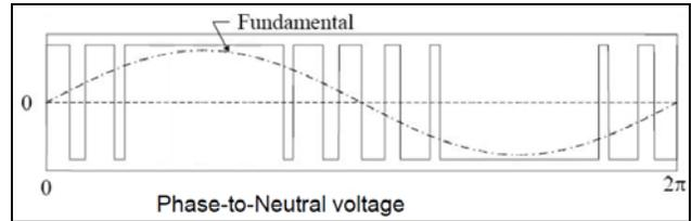
Figure 5 – 2-Level Switching
